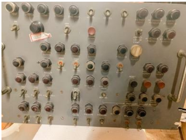
Electrical equipment panel I designed – it was used for Thor and Delta propulsion system testing, 1956-1970
